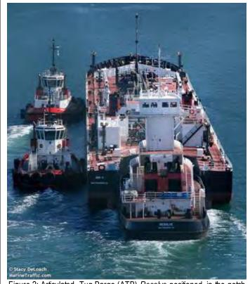
Figure 2: Articulated Tug Barge (ATB) Resolve positioned in the notch of its barge and made fast by a mechanical connection.
