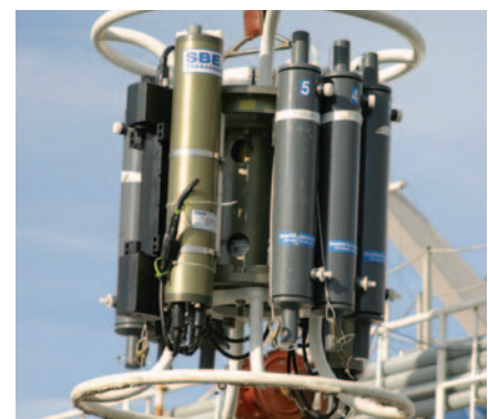
Figure 29. Water quality data is collected by lowering equipment into the ocean to sample a water column profile from the bottom to the surface. This rosette is a series of instruments on a metal frame that measures temperature, pressure, salinity, oxygen content, algae content and other factors, and features chambers to collect water samples at pre-determined depths.
